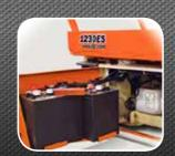
Serviceability All-steel swing-out battery doors have heavy-duty hinges.
